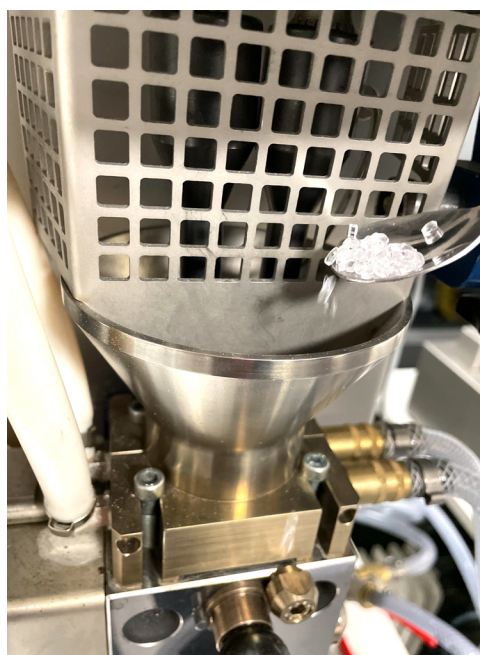
Figure 2. Both PET resin in pellet form and the chain extender in powder form added from the top water-cooled hopper of MC15 HT
