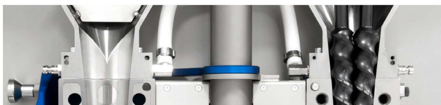
Figure 1. Forced feeding area of the intermeshing screws
