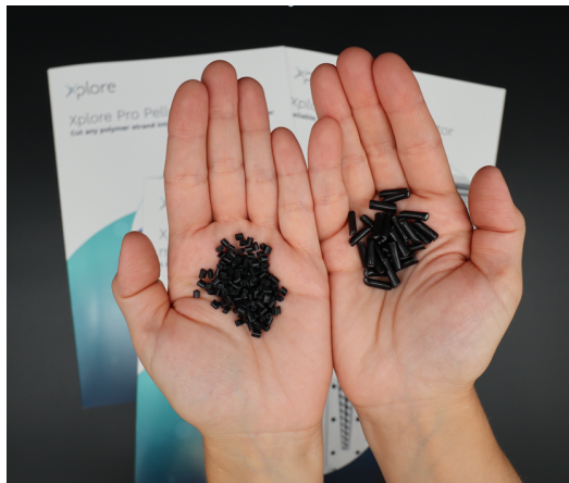
Figure 1. Short fiber (SF) reinforced (left) vs long fiber (LF) reinforced (right) pellets
